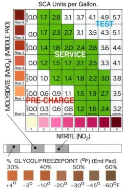
to the color chart and record result (be sure to use the bottom row on the chart if the result is white). (3) Finally compare NITRITE test to the color chart and record result. NOTE: The color chart to the right is a reference - your computer monitor or printer might not print colors accurately.
